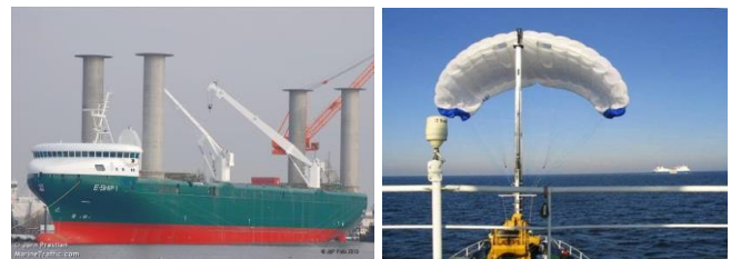
Wind-induced ancillary propulsion techniques (left: ©Jörn Prestien, right: seen on http://www.skysails.info/ , 05.05.2012)
